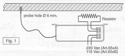
Connections have to be carried out by qualified persons following the diagram in fig.1. The resistor must have a maximum power of 2200 Watt with 220 Vac (Art.65xA) power supply and 1150 Watt with 115 Vac (Art.65xB) power supply. Class II device.
