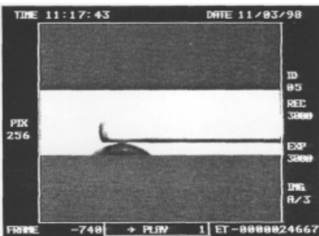
Fig. 3: The most surprising result: On just one miscue, the tip, the ferrule and even the shaft can all contact the cue ball.
